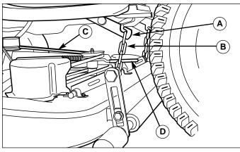
Figure 4. Mower Lift A. Lift Hook
